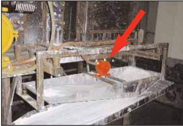
VS-320 SILENT TURBINE VIBRATOR ON PAINT SLURRY reduced surface tension and increased product flow significantly so paint no longer built up on slurry.
