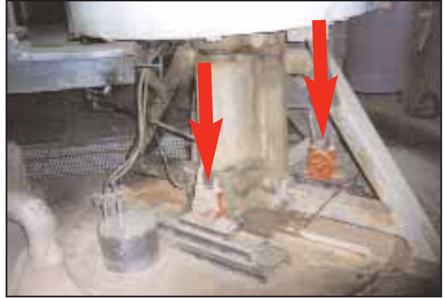
BVS-570 SILENT TURBINE VIBRATOR ON REACTOR WITH HEAT MOUNT keeps lead oxide from building up on the cover. Three tier special mount keeps vibrators from the heat and operating in critical application.
