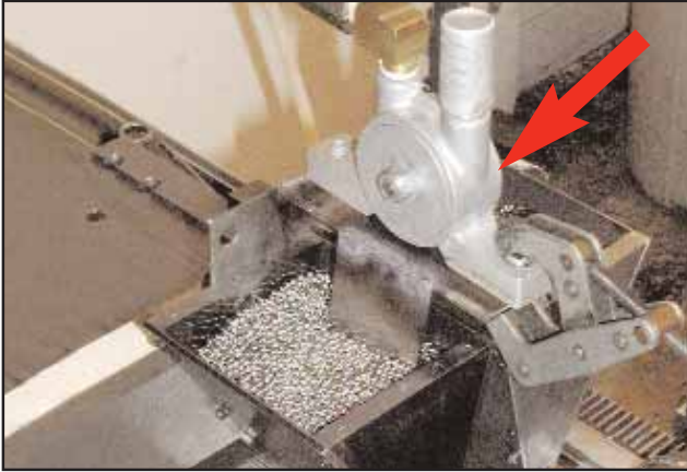
BVS-130 SILENT TURBINE VIBRATOR ON CHUTE produces a smooth flow of ball bearings to the feeder tray below.
