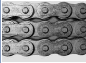
Neptune 700 Hours Salt Spray Test
