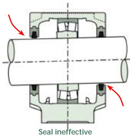
SRB units have inherent advantages over traditional solid bearing arrangements when considering sealing. The spherical location between housing and support ensures that whichever type of seal is used, it will always remain concentric to the shaft.
