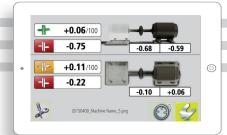
Rotate the sensors to 3:00, measure. The results will be displayed on screen.
