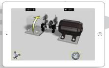
Rotate the sensors to the 12:00 position. Press the measurement icon again to take the second measurement.
