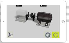
Rotate the sensors to the 9:00 position and press the measurement icon.
