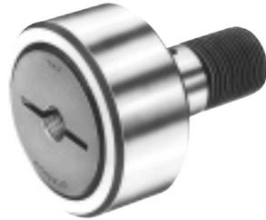
Basically the same as the popular type Cam Follower, this model is provided with tapped holes for piping on the stud head and the thread.
