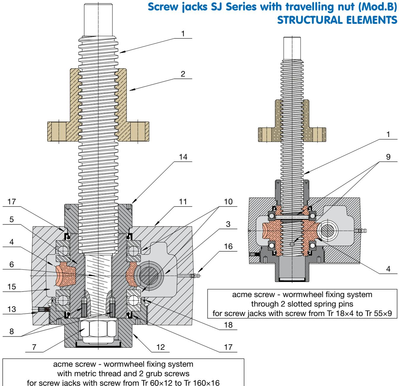
acme screw - wormwheel fixing system
