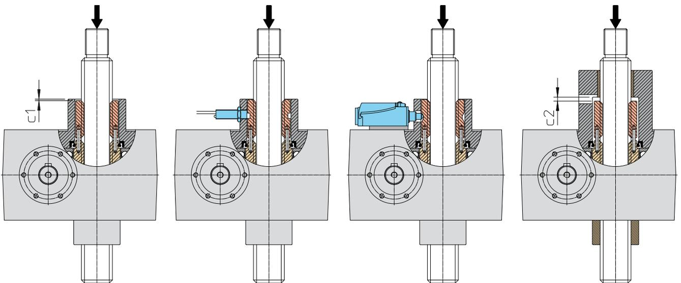
Thread wear control on screw jacks SJ Series Mod.A
