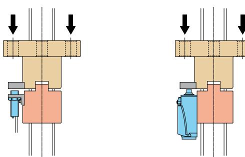
Thread wear control on screw jacks MA Series Mod.B
