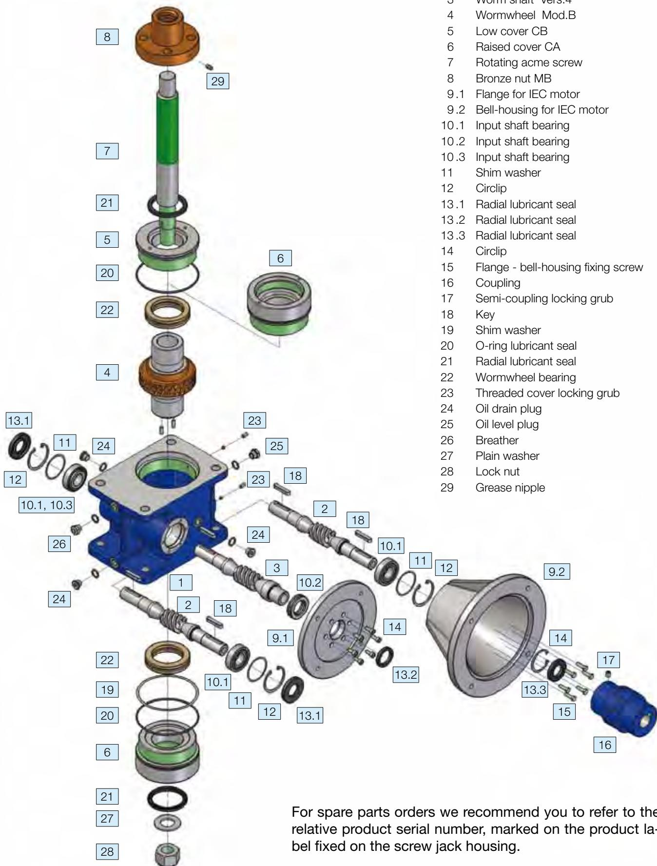
For spare parts orders we recommend you to refer to the relative product serial number, marked on the product label fixed on the screw jack housing.
