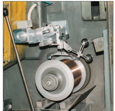
Non-contact flange detecting system with light barrier FA
