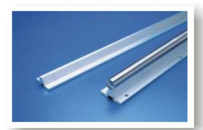
Shaft support Rails are designed to support the shafts on which ball bushings run to prevent them from bending under load.
