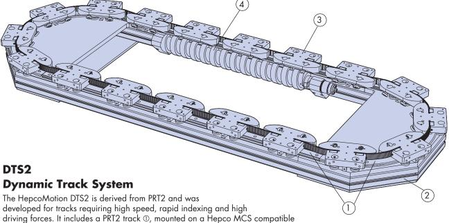
frame ②. Its carriages ③, are linked with adjustable spring-loaded belts and driven by a screw ④. The DTS2 can be supplied with motors, drives and bleed lubrication system ( 🚨 52). DTS2 units can be oval as illustrated, rectangular, or have any other valid track layout without S-bends. A range of sizes is available, in either standard or corrosion resistant version.
