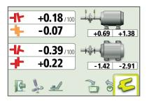
Rotate the sensors to the third position and measure. The results will be displayed on screen. Press the shim icon.
