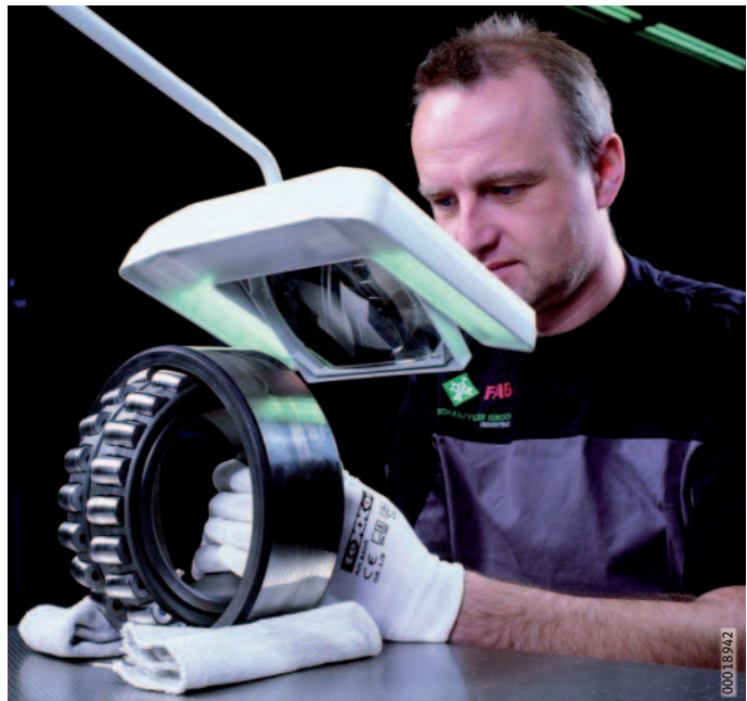
Figure 15 Bearing examination by Schaeffler reconditioning specialists
